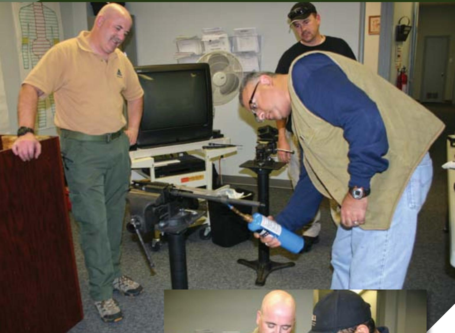
Removing troublesome gas block with aid of acetylene torch. ▲
