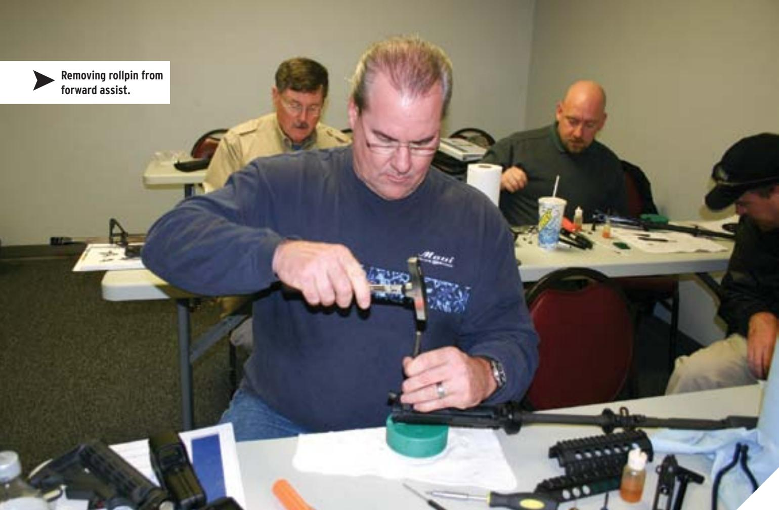
After going over basic fieldstripping early the first day, we graduated to detailed disassembly of the lowers and removed every subcomponent until we were left with bare lowers. Reassembly proved tricky, and Sully made sure to walk us through staking the castle nut of the receiver extension, aka buffer tube.
